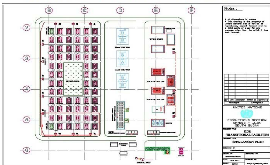
The layout of a transitional facility
